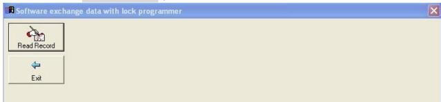
Connect the lock programmer, click "Read Record", upload the data from lock programmer to pc for view.
