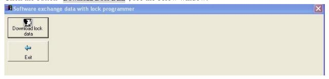
Connect the lock programmer, click "Download lock data", download the data from pc to lock programmer, finished downloading, confirm frame of "Download data success" was opened up, click "ok", you can use the lock programmer to download data to locks.
