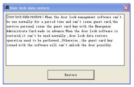
When the door lock management software can't be use normally for a period time and can't issue guest card ,the service personal issue the guest card key with the Emergency Administrate Card made in advance. When the door lock software is restored ,it can't be used normally ,door lock data restore operation need to be performed ,Otherwise ,the guest card key issued with the software will can't unlock the door possibly.
