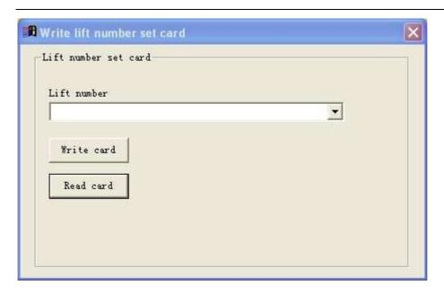
Select one lift number before making card, click "Write card", the Lift port setting card will record the mapping relationship of lift floor and controller port, the card should be run on the elevator, then use this card wipe the controller one time. .
